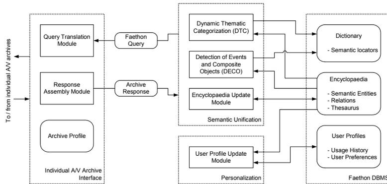
Figure 2. The FAETHON system at update mode of operation.
